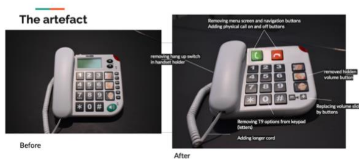
Figure 8 Picture memory phone before and after modifications
