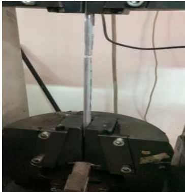
Fig. 8.B-Fracture point of Alpolic panel (max resistance) (Source:Authors)
