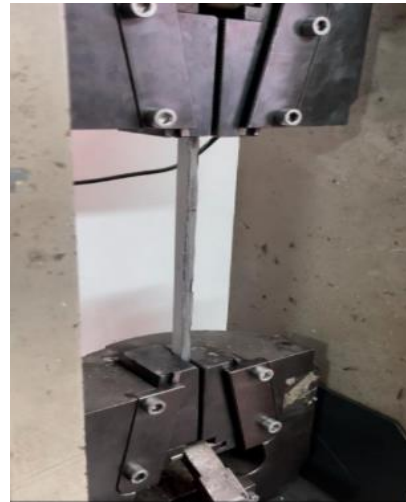
Fig. 7.C- Alpolic panel applied in the equipment (Source: Authors)
