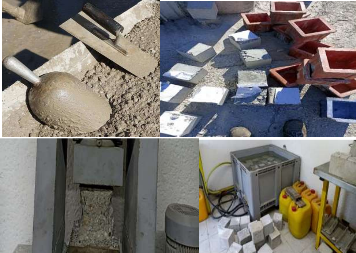
Figure 4. Tools and instruments used for sampling and compressive strength of concrete; source: authors
