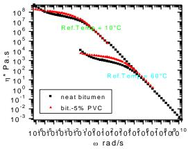
Figure 5: Master curves of  $\eta^*$  for bitumen and bitumen blends as a function of  $\omega$  at  $T_0=10$  and  $60^{\circ}C$
