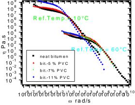
Figure 2: Master curves of  $\dot{\eta}$  for bitumen and bitumen blends as a function of  $\omega$  at  $T_0=10$  and  $60^{\circ}C$
