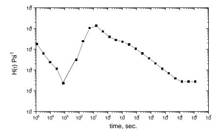
Figure 2: Plot of the relaxation spectrum for PVA 83K at  $T_0 = 25C$ .
