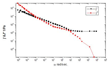
Figure 1: Master curve of the compliance for PVA 83K at  $T_0 = 25C$ .
