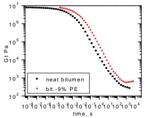
Figure 4: G(t) of bitumen/PE and neat bitumen at  $T_0 = 25^{\circ}C$
