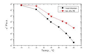
Figure 10:  $\eta^*$  of bitumen/PE and neat bitumen as a function of temperature at  $\omega = 0.1$  rad/s
