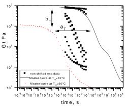
Figure 1: non shifted experiments data of G(t) at different temperatures are shifted into master curves at  $T_0 = 25^{\circ}C$  by using  $a_T$  and  $b_T$ .
