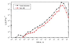
Figure 9: L(t) of bitumen/PE and neat bitumen at  $T_0 = 25^{\circ}C$
