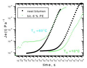
Figure 7: Je of bitumen/PE and neat bitumen at  $T_0$  = 10 and  $60^{\circ}\mathrm{C}$
