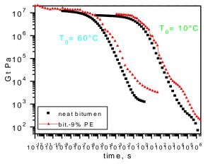
Figure 5: G(t) of bitumen/PE and neat bitumen at  $T_0 = 10$ and  $60^{\circ}C$
