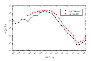
Figure 8: H(t) of bitumen/PE and neat bitumen at  $T_0 = 25^{\circ}C$
