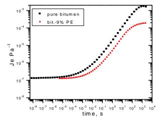
Figure 6: Je of bitumen/PE and neat bitumen at  $T_0 = 25^{\circ}C$
