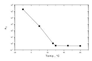
Figure 2:  $a_T$  of bitumen/PE blend as a function of temperature at  $T_0 = 25^{\circ}C$
