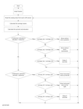
analog values from the light-dependent sensors. The next decision tests whether the average left is less than the average right. If the boolean logic returns True, this defines that there is no significant amount of sunlight present between the left and right portions of the system.
