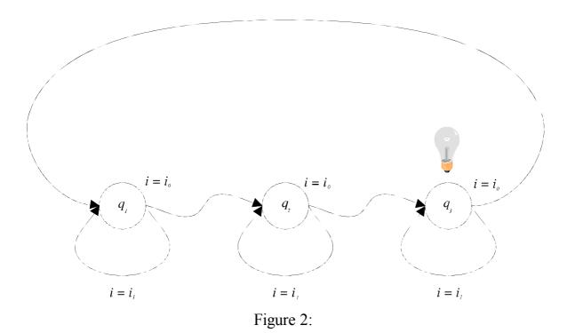
State transition Diagram of Turing's Wheel Machine - input undefined
