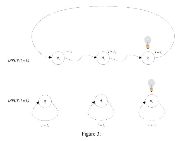
State transition Diagram of Turing's Wheel Machine – input defined
