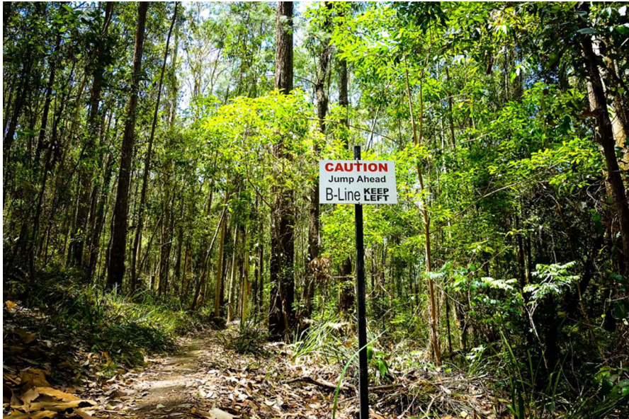
Fig. 1 Trail sign, Ourimbah cross-country mountain bike track. This sign prompts riders to prepare for the jump line on the right, or to veer left to avoid it. Importantly, it is placed on an unremarkable section of track, at eye height, to catch the rider's attention with enough time to make a decision about how to approach the upcoming section of trail, without having to stop riding in order to do so. Photo by Kath Bicknell.
