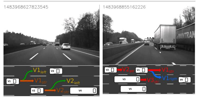
Fig. 2 Top: Screenshot of a Cut-In scene. Bottom: Birds-eyeview representation of the traffic situation and the behavior options for the autonomous vehicle V1 and the relevant other traffic participant V2
