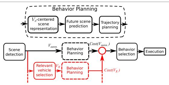
Fig. 1 The figure shows the processing flow of the driver assistance system. Black parts are shared between *ego* and *fair* behavior selection, red modules are only used in the latter. For the *fair* system, the planning module is run for every vehicle  $V_x \in \{V_1, ..., V_n\}$  in the surrounding and behavior selection is done using all individual costs, whereas the basic variant only considers the cost of the own trajectory ( $V_x = V_{auton.}$ )
