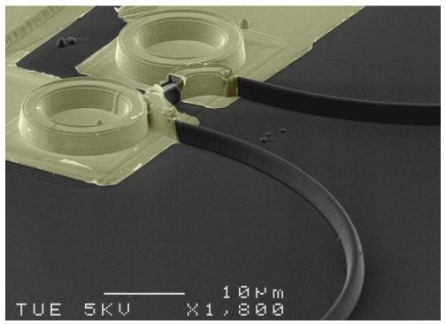
Fig. 1: Electron microscope picture of an optical flip-flop based on ring resonators with < 18 ps switching time. The device has been fabricated at TU/e<sup>10</sup> and occupies approximately 60 x  $40 \ \mu m^2$ .
