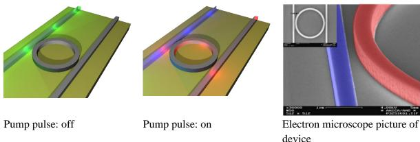
Fig. 2: Optical switch based on ring resonators with < 1 ps switching time<sup>11</sup>. The device has been designed and characterized by UT in cooperation with the RWTH Aachen and occupies
