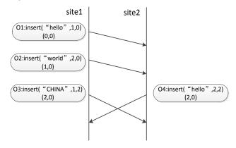
Fig.4 Insert string into different strings
