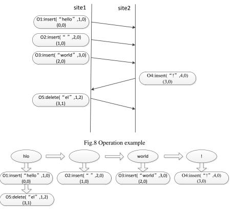
Fig.9 diagram of operation storage
