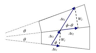
*Figure 18.* Point-motion on a cone. We can determine the x-acceleration of a straight-line motion geometrically, from first principles.
