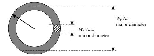
Figure 7. Geometry of the micro-torus.
