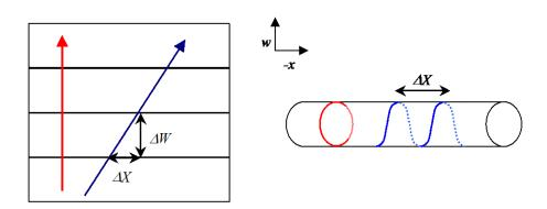
**Figure 16.** Geodesic point-motion on a pipe. The increment  $\Delta x$  in the *x*-direction is constant with each rotation. Neither trajectory is accelerating. Both trajectories are geodesics. Note we take the negative *x*-direction to be to the right.
