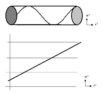
Figure 9. A line on a cylinder developed into a plane.
