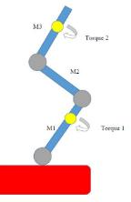
Figure 1 the triple pendulum
