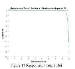
As we seen from the Figures above the angular displacements and the angular velocities are unstable.
