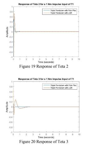
As we seen from Figure 18, 19 and 20, for the impulse signal the angles starts to increase and returns to zero degree for the two controllers but the pendulum with LQR controller has a high overshoot with more settling time than the pendulum with pole placement controller.
