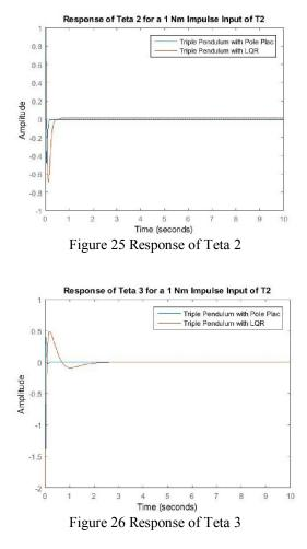
As we seen from Figure 24, 25 and 26, for the impulse signal the angles starts to increase and returns to zero degree for the two controllers but the pendulum with LQR controller has a high overshoot with more settling time than the pendulum with pole placement controller.
