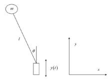
Figure 1 Vertically moving base inverted pendulum system
