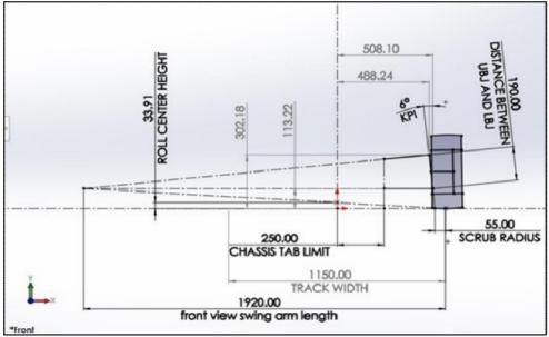
Fig. 2. Front view swing arm line diagram
