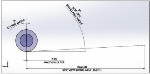
Fig. 3. Side view swing arm line diagram
