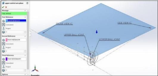
Fig. 5. Plane creation from Ic's and ball joints
