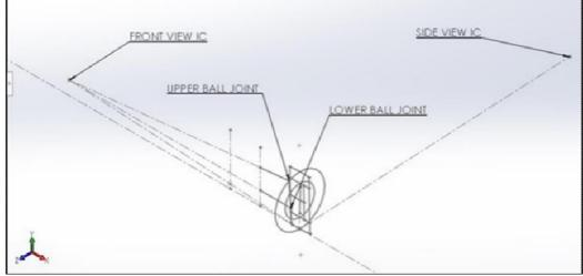
Fig. 4. 3D view of Instantaneous centres and ball joints
