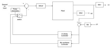
Figure 2: water level of the tank system with H  $\infty$  and  $\mu$  - synthesis controllers system interconnections block diagram for tracking level h1
