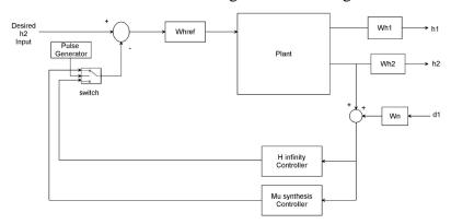
Figure 3: water level of the tank system with H  $\infty$  and  $\mu$  - synthesis controllers system interconnections block diagram for tracking level h2
