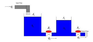
Figure 1 two-tank liquid-level control system
