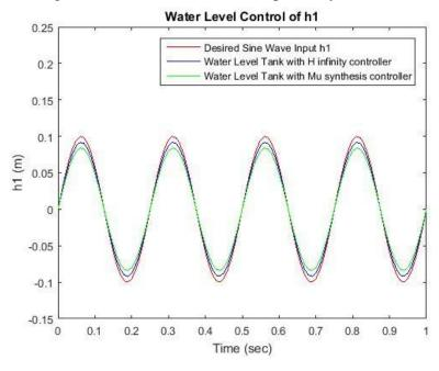
Figure 6: Simulation of the actual and desired level for h1
