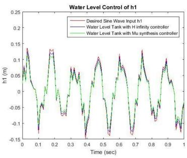
Figure 8: Simulation of the actual and desired level for h1
