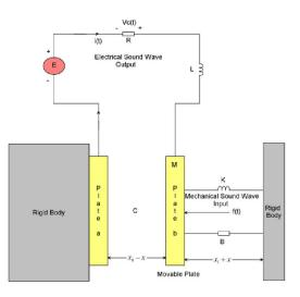
Figure 2 Capacitor microphone system
