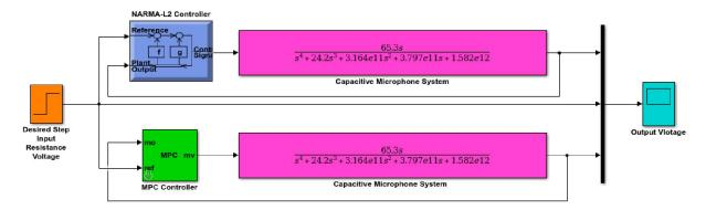
Figure 5 Simulink model of the capacitor microphone system with NARMA-L2 and MPC controllers for step desired sound waves voltage input signal
