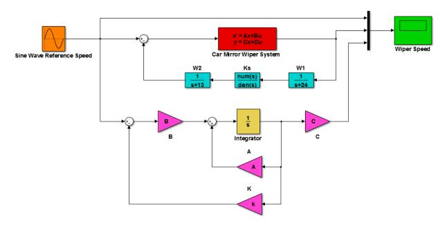
Figure 6 Simulink model of the vehicle windshield wiper system using H infinity loop shaping and robust pole placement controllers for tracking the sine speed reference
