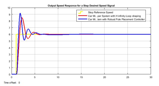
Figure 5 Simulation result for a step reference input
