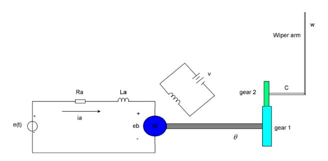
Figure 1 Electromechanical car mirror wiper system
