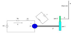
Figure 1 Electromechanical car mirror wiper system
