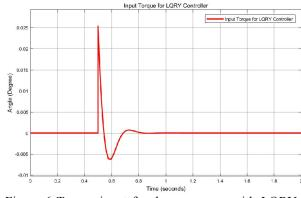
Figure 6 Torque input for the gyroscope with LQRY controller
