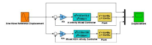
Figure 6 Simulink model of the solenoid based linearly movable armature system using H infinity mixed-sensitivity and mixed H  $_2$  /H $_\infty$  with regional pole placement controllers for tracking the sine wave references displacement signal
