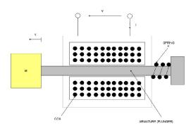
Figure 1 Solenoid based linearly movable armature system
