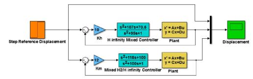
Figure 4 Simulink model of the solenoid based linearly movable armature system using H infinity mixed-sensitivity and mixed H 2 /H\infty with regional pole placement controllers for tracking the step references displacement signal
