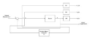
Figure 2 Solenoid based linearly movable armature system with H infinity mixed sensitivity controller block diagram
