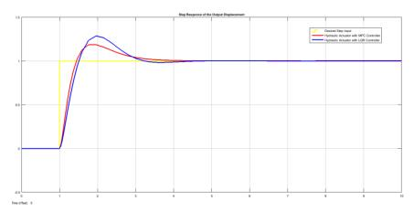
Figure 5 simulation result of the hydraulic actuator system with MPC and LQR controllers for a step desired input signal
