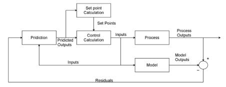
Figure 3 Block diagram for model predictive control.
