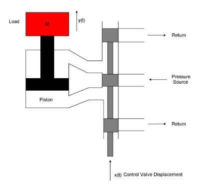
Figure 1 the hydraulic actuator system
