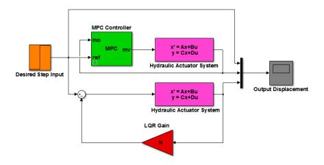
Figure 4 simulink model for the hydraulic actuator system with MPC and LQR controllers for a step desired input signal
