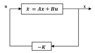
Figure 2 State variable feedback configuration
