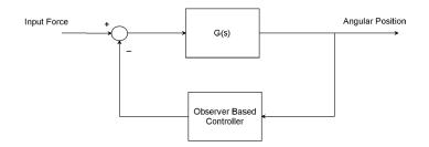
Figure 2 Block diagram of the inverted pendulum on a cart with the observer-based controller
