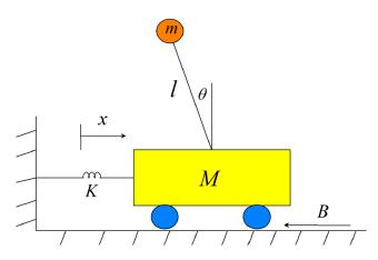
Figure 1 Inverted pendulum on a cart system model
