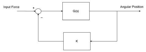
Figure 4 System with full state feedback H2 controller
