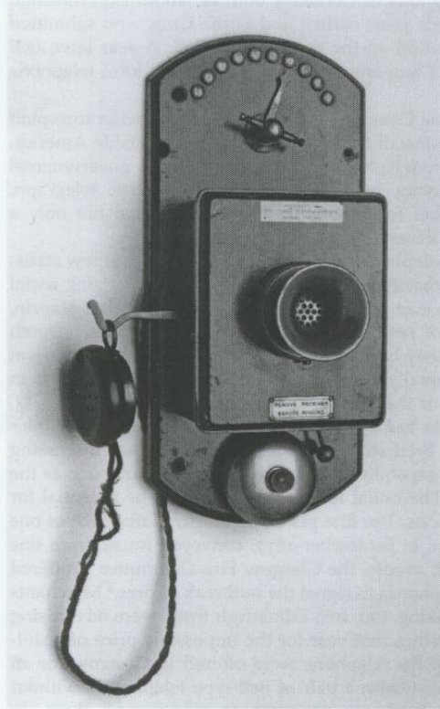
Figure 26.1 An intercommunications telephone, Peel Conner, 1904. It has a selector dial for ten internal lines. NMS T.2003.265.
