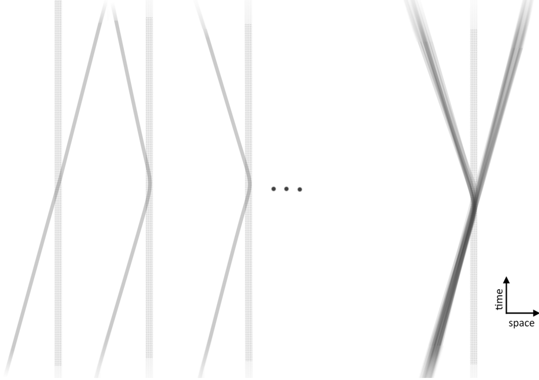
Figure 1: BU time slices (left) allegedly involved in a single-particle—Q M experimnt. Thick vertical lines represent a crystal lattice. Thin grey lines are initially left-to-right moving particles, some transmitting, others reflecting. By ‘superimposing’ all members of the ensemble (right), one gets various ensemble densities, e.g. charge density \rho_{\text{ens}} , from which the (statistical) results of any Q M experiment can be deduced. From the constraints satisfied by individual members in the ensemble, equations for the ensemble densities can be derived [3], and, upon writing \rho_{\text{ens}} \equiv \phi^\dagger\phi , Q M wave equations for \phi follow. Different \phi ’s then describe different ensembles rather than any single system (hence Ehrenfest’s theorem, ‘scars’ and general amplitude amplification of wave-functions near classical periodic orbits, and the inevitable rapid wave-function delocalization of manifestly macroscopic but chaotic systems[9]). The NG nature of the Schrödinger evolution is a consequence of local energy-momentum conservation, rather than being a property of individual systems. Note that different members are brought to a common time support so the Schrödinger evolution is fictitious—a mathematical tool for constructing ensemble densities; ensembles representing steady-state systems even correspond to multiple time slices of a single system. The construction in [3] only works for closed systems, hence the Hamiltonian. And indeed, when a closed system becomes coupled to the environment, as must be the case during its ‘measurement’, the initial wave-function and its evolution become nonsensical. Distinct ensembles, represented by distinct wave-functions, \phi_m must then be defined post measurement (insofar as Q M is to be subsequently applied) and the collapse postulate is just that complementary statistical ingredient, bridging the pre-post measurement gap, giving weights to different \phi_m ’s based on their corresponding macroscopic ‘pointer configuration’. Heisenberg’s uncertainty relations, reflecting certain properties of ensembles, are in line with the role of an agent in the BU, i.e., that its action—measurement in this case—defines an ensemble.
