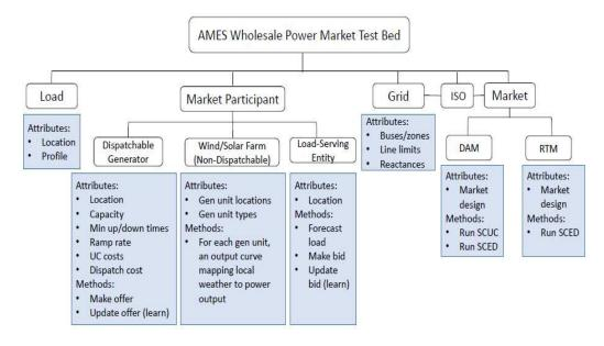
Figure 6: ACE computational platform permitting study of U.S. ISO-managed wholesale electric power markets. Source: Tesfatsion (2017j).
