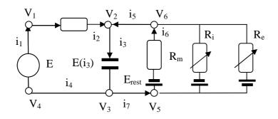
Figure 14 Electrical scheme for shunting inhibition.  $R_e$  is the excitatory resistance,  $R_i$  is the inhibitory resistance,  $R_m$  is the resistance of the membrane.
