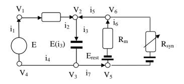
Figure 12 Electrical circuit for synapses.
