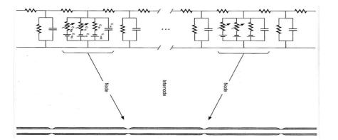
Figure 10. Axons with myelin and electrical circuit
