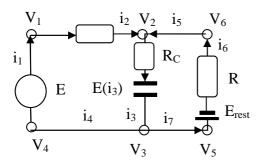
Figure 3 Membrane resistances and equivalent electrical circuit
