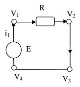
Figure 2 Toy electrical circuit with one generator E and one resistor R
