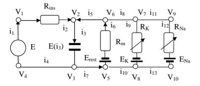
Figure 7 Electrical membrane circuit with voltage-gated channels in the membrane
