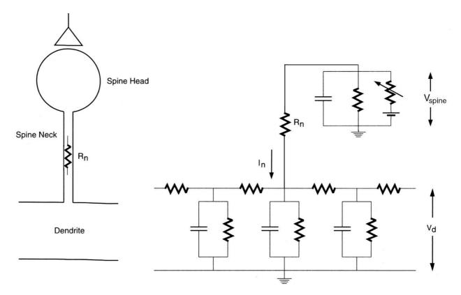
Figure 13 Electrical connection between synapses and dendrite.
