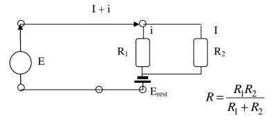
Figure 4 random  $R_1$  and crisp resistance  $R_2$  generate the equivalent resistance R in a parallel configuration.
