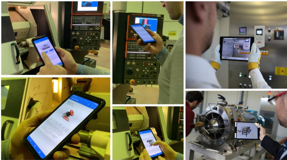
Figure 13. Prototypes of voice-enabled digital assistants that augment the worker's interaction capabilities towards the CPPS.
