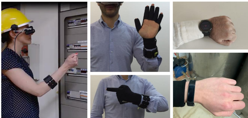
Figure 9. Example of wearable technology—from left to right, wristbands, gloves, smartwatches—augmenting workers' perception capabilities.
