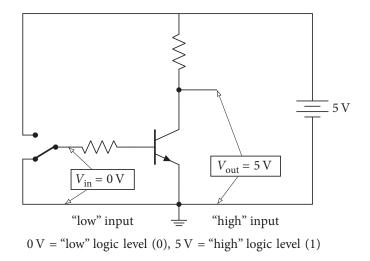
Figure 13.1 A state flipper (transistor in cutoff)
