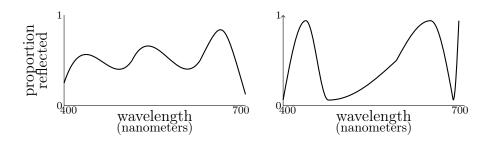
At least in principle, objects can reflect light in infinitely many different ways, because they can reflect different proportions of light at any of the infinitely many wavelengths between 400nm and 700nm. As a result, there are a great many ways in which we could rank objects by how they reflect
