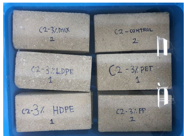
Fig. 2 The prepared cement bricks were cured in the water for 28 days
