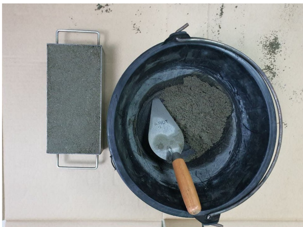
Fig. 1 The casting process of cement brick containing plastic aggregate
