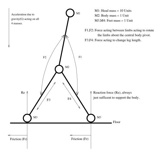
Figure 6.1: The Physical Configuration of the Bipedal Machine
