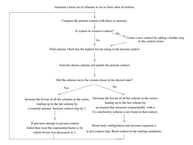
Figure 9.1: Flowchart Representation of the First Program.
