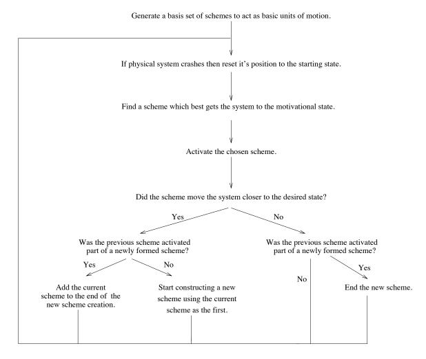
Figure 8.1: Flowchart Representation of the Preliminary Program
