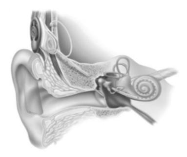
Fig. 9.1 A commercial cochlear implant device consisting of an extracorporeal sound processor with a microphone and an attached transmitter coil that relays signals through a radio link to the receiver unit connected to the intracochlear electrode array inserted into the cochlea (Source: Kral et al. 2004).
