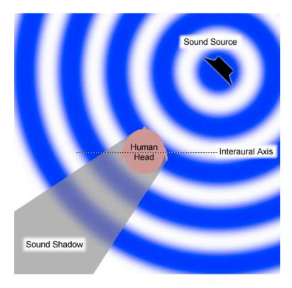
Fig. 7.1 A sketch showing the shadowing of a sound source by the head and a depiction of interaural phase difference. The circles mark contours of constant phase. (Source: Perrett, 2009)
