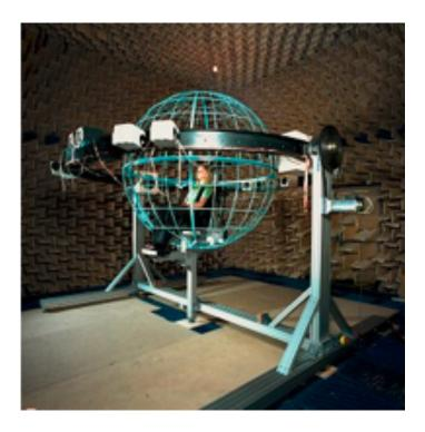
Fig. 7.3 Apparatus used at the University of Southampton Institute of Sound and Vibration Research to investigate sound direction localization. (Source: Virtual Acoustics and Audio Engineering, University of Southampton)
