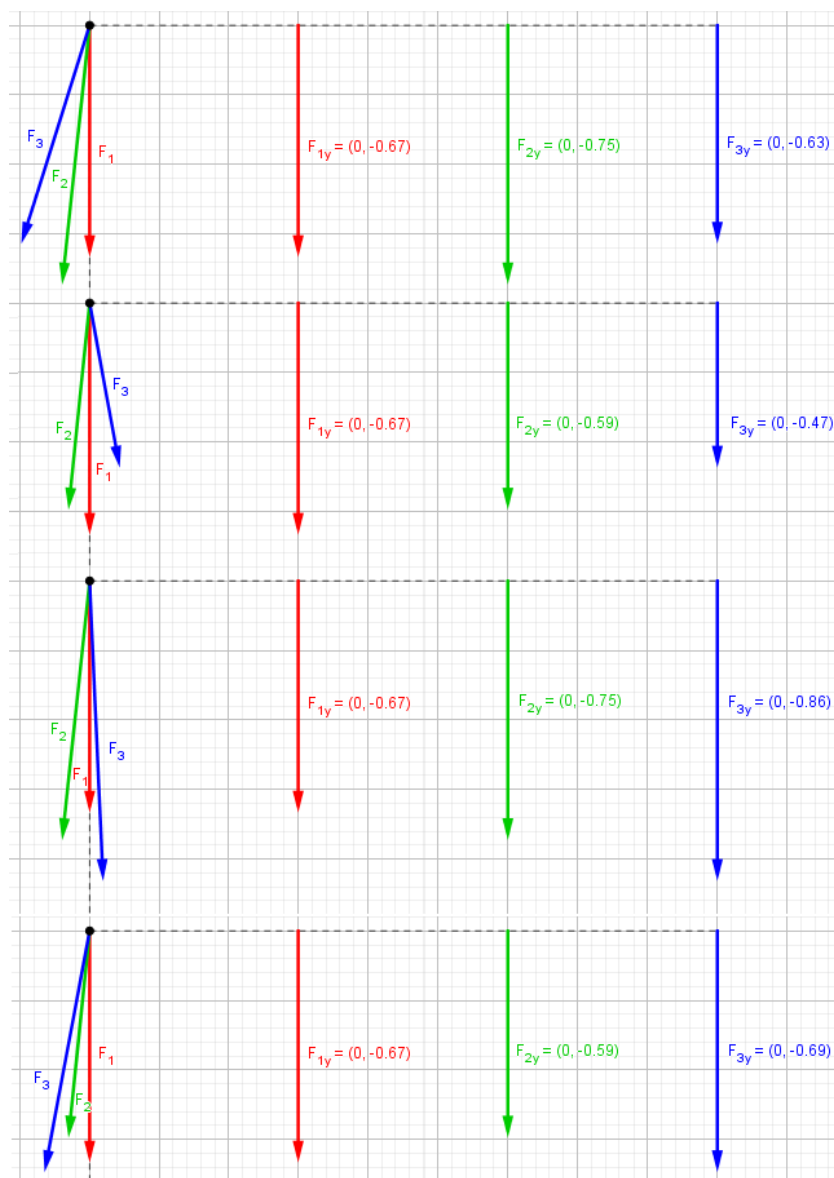
Figure 14: The dynamic vector diagram of Y-component F_y of the resultant of the forces acting on the body in four cases (from top to right): t_i = 0, rot = 1 ; t_i = TM, rot = 1 ; t_i = 0, rot = -1 ; t_i = TM, rot = -1 .
