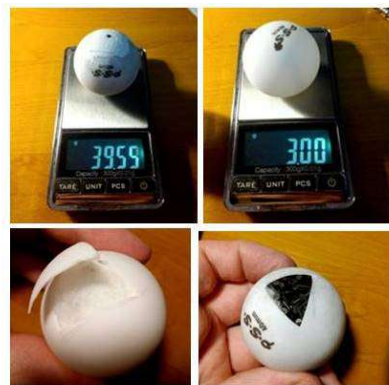
Figure 7: Manufacture of balls to measure the acceleration of free fall.
