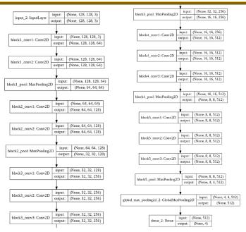
Figure 5 Architecture of VGG 16 model
