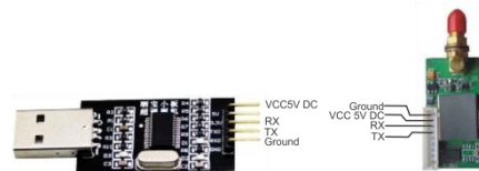
Fig 3. USB to RS232 TTL PL2303HX converter configuration
