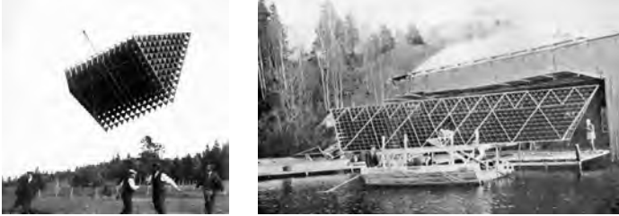
Alexander Graham Bell. Left Early tetrahedral kite. Right A later, much larger version of the same configuration called the "Cygnet" (1907).
