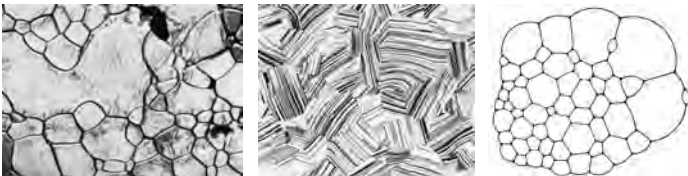
Left Aluminum alloy structure after heating, from Cyril Stanley Smith (1957). Middle Copper-silicon alloy structure. Right Foam structure ("soap froth").
