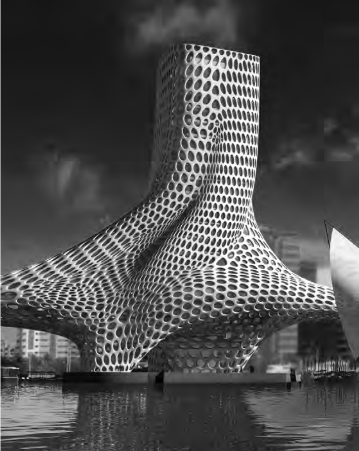
NOX, The Three Graces, Dubai (2008). Detail showing the hotel tower, one of in total three towers standing at the end of the piers of the Khor Dubai Wharfage, interconnected by a footbridge. The structural skin consists of an aggregate of deformed lattices; where the lattice is made purely of hexagons, the jumps in the aggregate are produced by pentagons, heptagons and other polygons. See also "Textile Tectonics", p. 236–7, and "Steel and Freedom", p. 266–7.
