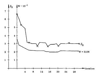
Figure 3. Iteration history for failure defined at level 2. × indicates identification of significant failure modes.
