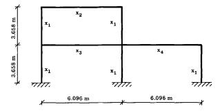
Figure 2. Geometry and optimization variables.
