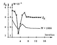
Figure 4. Iteration history for failure defined at mechanism level.  $\times$  indicates identification of significant failure modes. The NLPQL algorithm is used.
