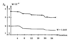
Figure 8. Iteration history for failure defined at mechanism level. X indicates identification of significant failure modes. The NLPQL algorithm is used.
