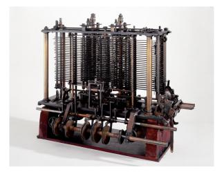
Figure 2. Babbage's Analytical Engine.
