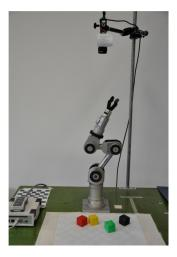
Figure 2. The Katana robot arm. Source: Ngo 2012.
