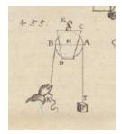
Figure 1. Diagram of a fixed pulley. Source: SCHOTT 1661.
