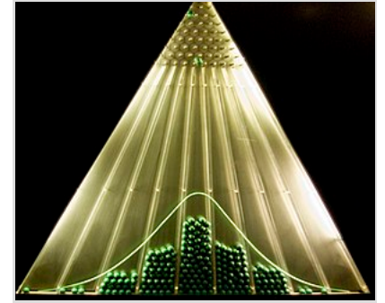
The bean machine , designed by early social research methodologist Sir Francis Galton to demonstrate the normal distribution , which is important to much quantitative hypothesis testing [a]
