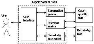
Figure 1: Architecture of an Expert System
