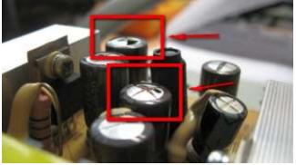
Figure 4: The figure shows the Power Supply Failure [3]
