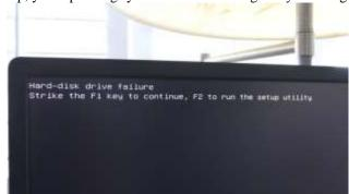
Figure 5: The figure shows the hard disk failure in desktop PC [6]
