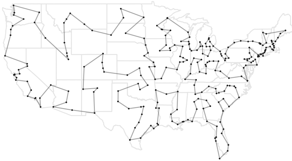
Figure 3: The output of an optimisation process, which reduced the path length to 20891 miles.
