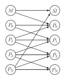
Figure 2. Proposed DAG for the differential model. The dots on the variables indicate time derivatives.
