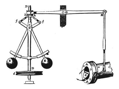
Figure 28.1 Watt's centrifigual governor for a steam engine
