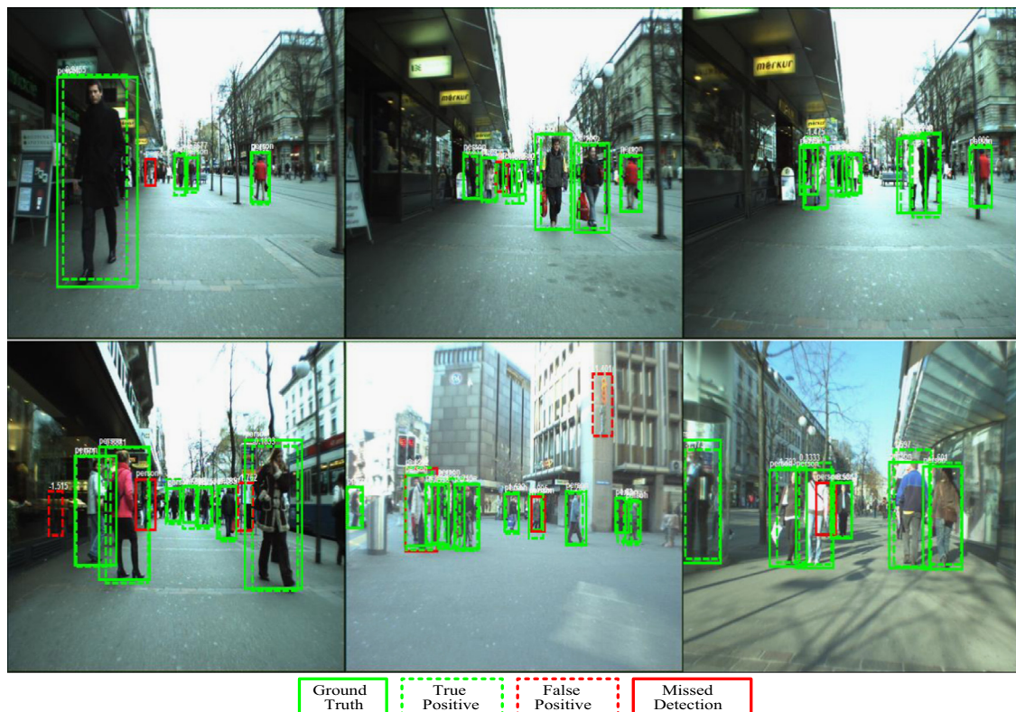
Fig. 7. Detection results using our hierarchical structure model on the ETHZ dataset. (The green dotted bounding box means correct detection; the red solid bounding box is missed detection; and the red dotted bounding box is false positive.) (For interpretation of the references to color in this figure legend, the reader is referred to the web version of this article.)
