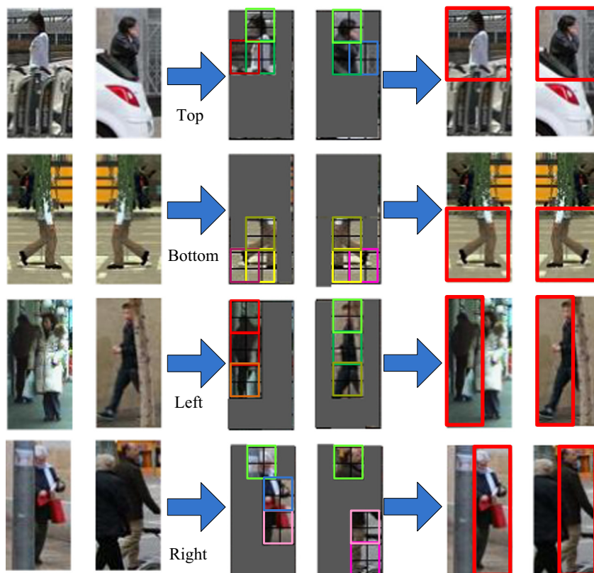
Fig. 1. Complex occlusion patterns and estimation of visibility of a part from its detection score or from its correlated components. Black regions represent the estimated parts that are not visible.
